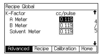
Fig. 36. Advanced Setup Screen 4
